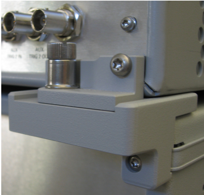
Figure 9 Locking Feet Screws
