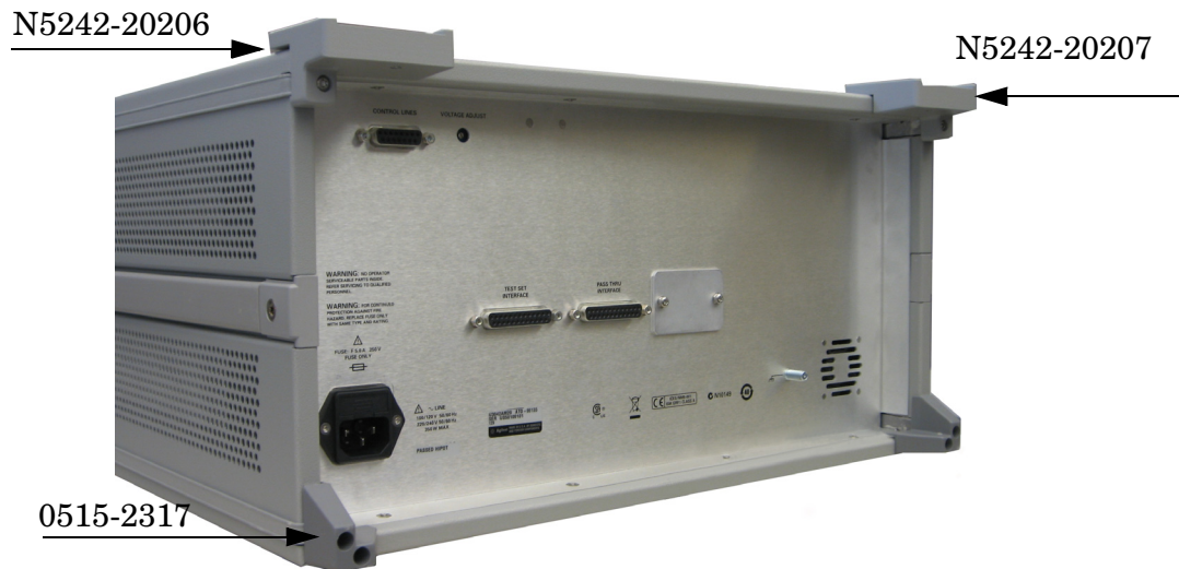
Figure 7 Install Locking Feet on Test Set
